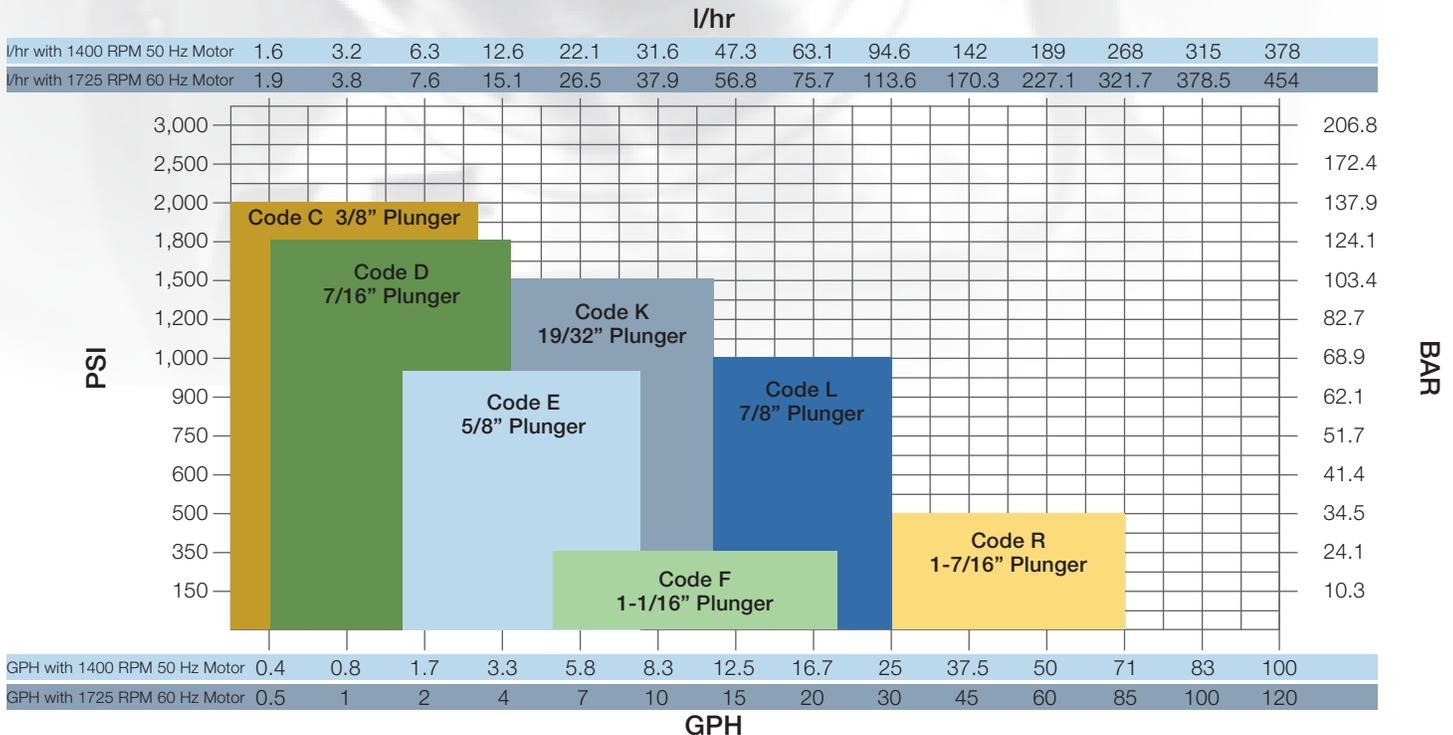
\*Values are for simplex pumps only. For duplex configurations, the pressure will not change, but the capacity values will double.
